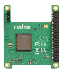
**Radxa 20W PoE+ HAT** is a high-efficiency power supply solution designed for Single Board Computers (SBCs). It complies with IEEE 802.3af/at PoE standards, supporting power and network transmission through a single cable, significantly simplifying device wiring.
