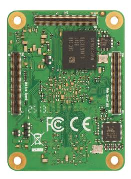
Radxa CM4 is a high-performance system-on-module designed to bring the capabilities of the RK3576 processor to space-constrained and custom embedded applications. Built around a  $55 \text{ mm} \times 40 \text{ mm}$  compact form factor, CM4 is ideal for industrial control, edge computing, computer vision, and multimedia applications.
