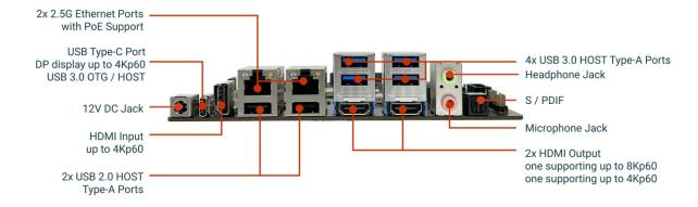
Note: The actual board layout or components' location may change during the time but the main connectors type and location will remain the same
