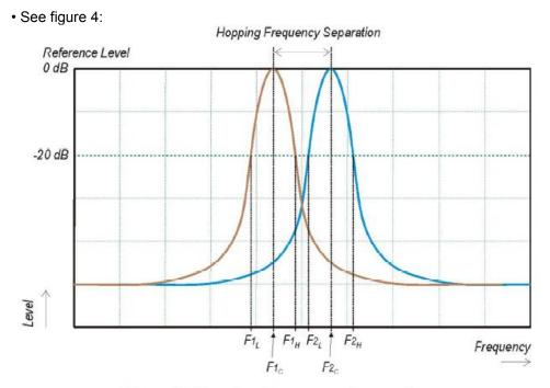
Figure 4: Hopping Frequency Separation
