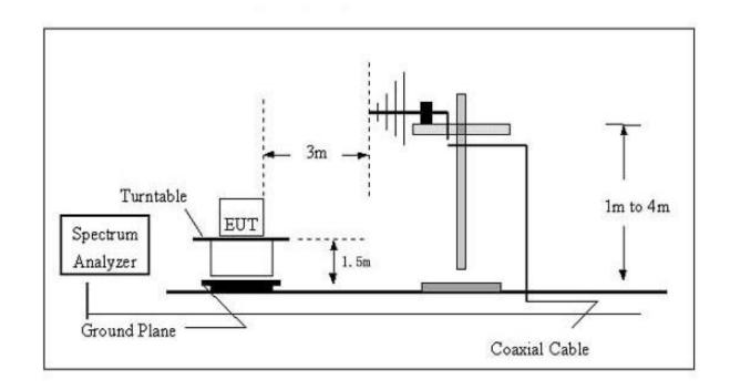
(B)Radiated Emission Test Set-Up Frequency Above 1GHz.
